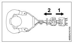
The MultiEngine with rotor blades can be operated forwards (1) or backwards (2).
