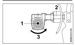
Gearbox output shaft (1) below the drive tube (2).
