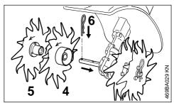
Rotate the inner right-hand blade (4) on the shaft until it can be pushed into position – check the direction of rotation again (arrows).
